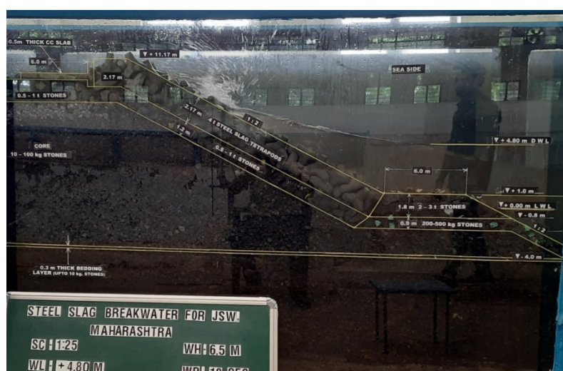
Wave Flume Studies for the Confirmation of Hydraulic Stability of the Structures by using Steel Slag
