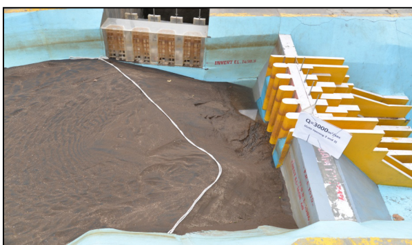
Formation of distinctive scouring cone for gate 2 & 3 open condition and Q = 3000 \text{ m}^3/\text{s}
