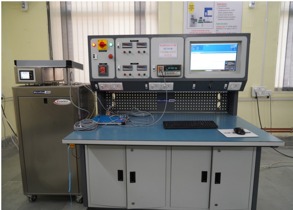
Air temperature sensor calibration system
