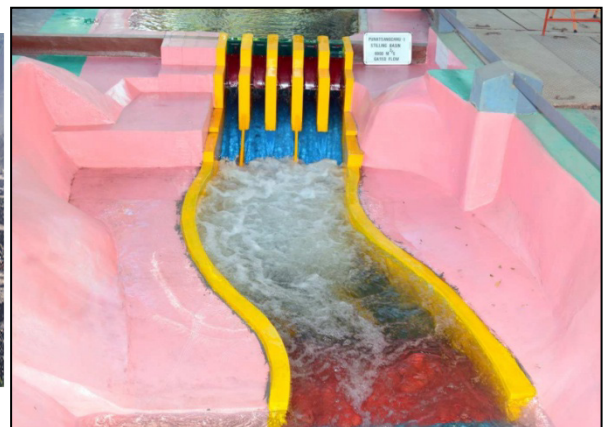
Flow conditions downstream of the spillway
