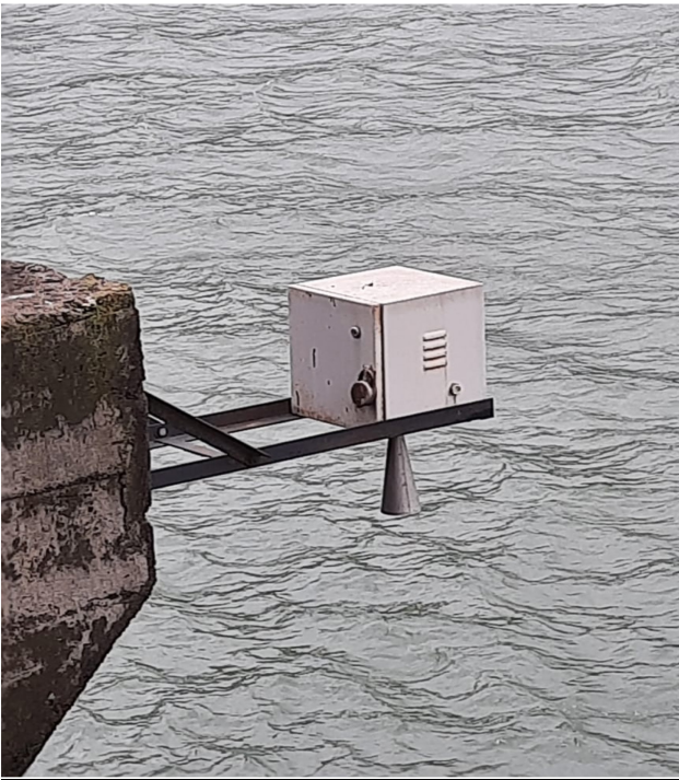
Field inspection of AWS and AWLR, installed at Koynanagar, Satara by Water Resources Department (WRD), Maharashtra
